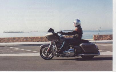
benefits from all of the Project Rushmore enhancements, including a new 49mm fork, Reflex linked brakes, sleeker fenders, One-Touch bag latches and vents, lighter cast wheels, improved hand controls, instrumentation and comprehensive infotainment systems.
