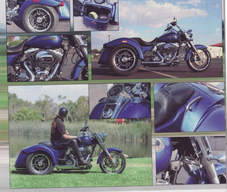
toggle button on the left controls and an "R" lights up in the Speedo. Then press the R button again and you're moving in reverse. It's not designed to back you up a hill, just to get you out of parking spaces. The Freewheeler won't start unless you're in neutral, you can't just grab the clutch and hit the starter.
